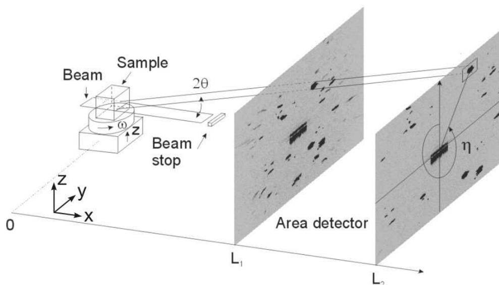
Figure 6.7.2: Grain mapping of a polycrystalline material by 3DXRD (courtesy H.F. Poulsen)
