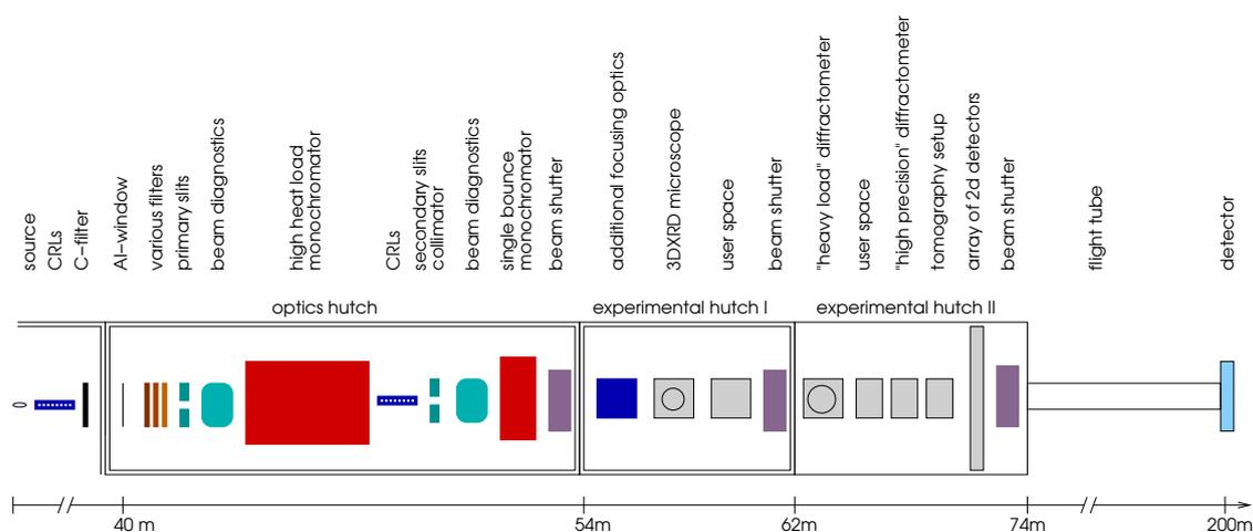
Figure 6.7.4: Schematic layout of the high energy materials science beamline.
