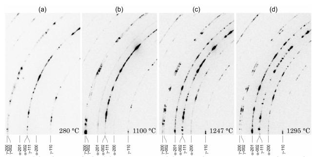
**Figure 4:** Selected extracts of Debye-Scherrer patterns recorded in-situ at the given temperatures upon heating. The transformation from massively transformed  $\gamma$ -phase (a) through the  $\gamma + \alpha$ -field (b,c,d) close to  $T_{\alpha}$  is clearly seen and shows many features along the rings.
