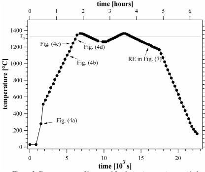
**Figure 3:** Temperature profile as used for the in-situ experiment with data acquisition points, full circles. The tags relate to Figs. (4) and (7). RE marks the evaluated point after re-entrance into the  $\alpha + \gamma$ -field from above  $T_{\alpha}$ .
