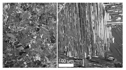
Figure 2: Microstructure of the sample before a) and after b) the heating cycle as shown in Figure (3). The massively transformed starting material recystallizes into a fully lamellar structure.
