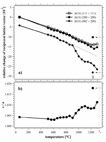
**Figure 7:** Temperature dependence of (a) reciprocal lattice vectors and (b) c/a ratio of the  $\gamma$ -phase. The arrows mark the data points RE, see Figure (3), after re-entering the  $\gamma + \alpha$ -phase field from above  $T_{\alpha}$ .
