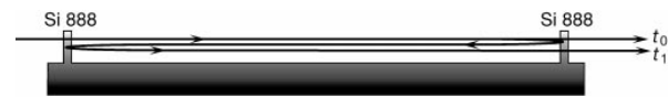
Figure 1 Sketch of the resonator with the two active slices sticking out of the monolithic device. Photons impinging from the left can be trapped due to transmission and reflection probabilities T and R , respectively. They exit the resonator with probabilities TT , TRRT , TRRRRT \dots T^2R^{2N} for 0, 1, 2, \dots, N back-and-forth bounces at t_0, t_1, \dots , being delayed by N times the time of flight inside the resonator of 1.0 ns. The reflection angle is adjusted to exactly 180 degrees and the beam paths of multiply reflected photons are exactly superimposed in space.
